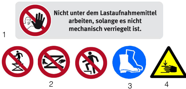
Fig. 1: Safety labels: 1 Prohibition sign with reference I 2 Prohibition sign I 3 mandatory sign Wear safety shoes I 4 Warning of danger of crushing the upper limbs
